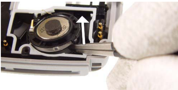
36.) Use tweezers as a lever when removing the IHF-Speaker .
