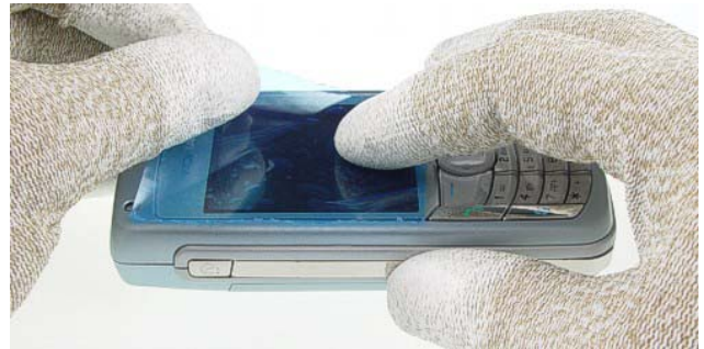
1.) Protect the window with a film.
