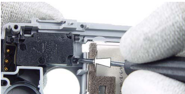
38.) Unlock the snaps with a slotted screwdriver carefully.
