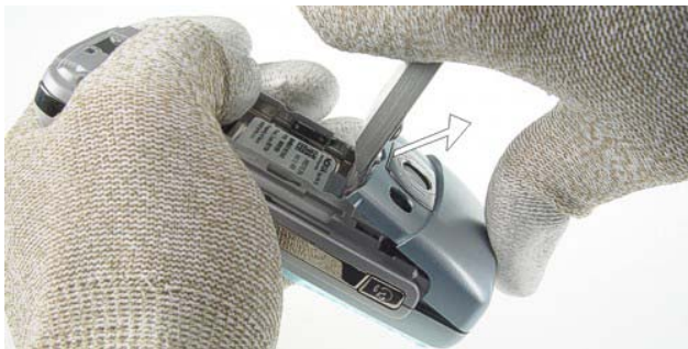
4.) Pull up the Antenna Cover carefully.
