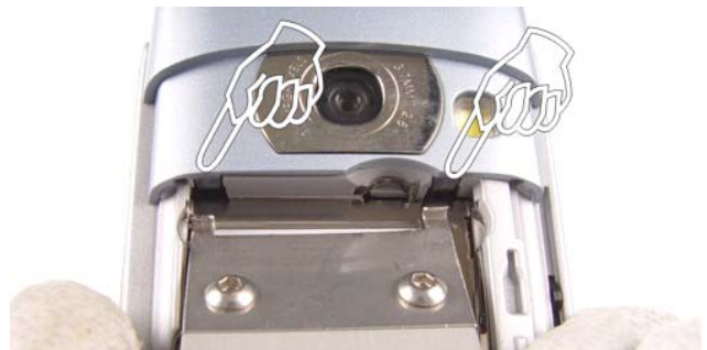
3.) Place the SS-68 into the openings.
