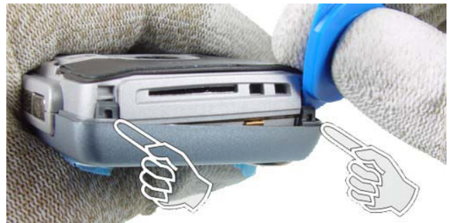
5.) Release the booth clips of the A-Cover with SRT-6.
