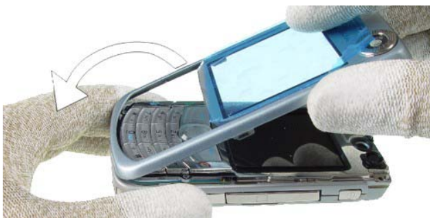
6.) Remove the A-Cover by turning it as shown in the picture carefully. Replace the A-Cover if it is necessary.
