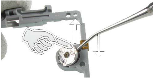
16.) Use the dental tool as a lever to remove the Earpiece.
