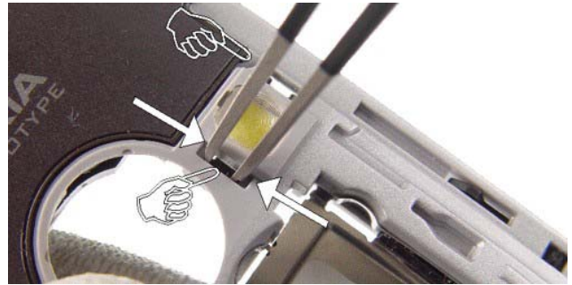
33.) Use tweezers to unlock the snaps of the LED Flash Holder .
